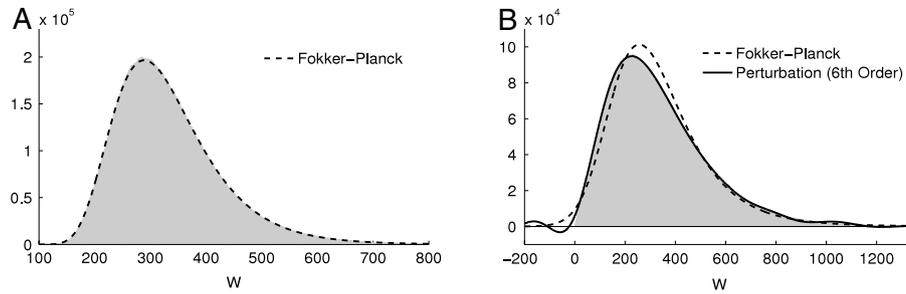
**Fig. 1.** Equilibrium distribution of weights from Monte-Carlo (shaded histogram) and as predicted by the FPE using (A) parameters from van Rossum et al., and (B) parameters for which the FPE fails. Also shown is the perturbation solution using terms through sixth order.
