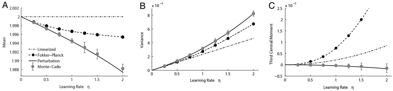
**Fig. 4.** Moments of the equilibrium distribution for ELL synaptic weights vs. learning rate. Shown are the moments calculated with the linearized theory, with the FPE, with the perturbation analysis and from Monte-Carlo simulations ( $\pm 2\sigma$  confidence intervals). (A) Mean to 4th order in perturbation, (B) Variance to 6th order in perturbation, (C) Third central moment to 4th order in perturbation.
