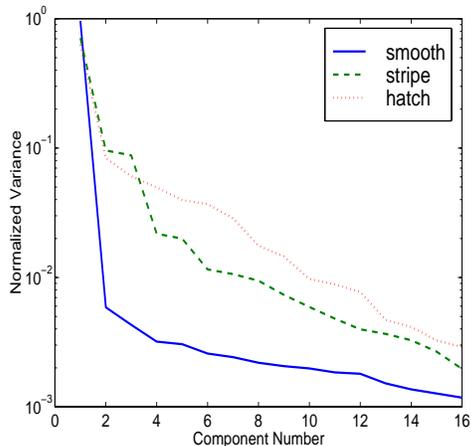
Figure 1: The three regions in the example image delineated by squares have vastly different correlation eigen-spectra. Assigning dimension by a fidelity requirement that places an upper bound on distortion would find a different dimensionality for each region.
