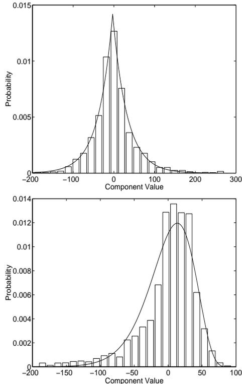
Figure 3: Coefficient value histograms and model densities: Laplace (top) and Pearson (bottom)
