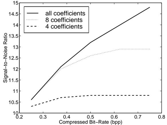
Figure 4: Quality of constrained vs. unconstrained bit allocation for compression using 128 region partition.
