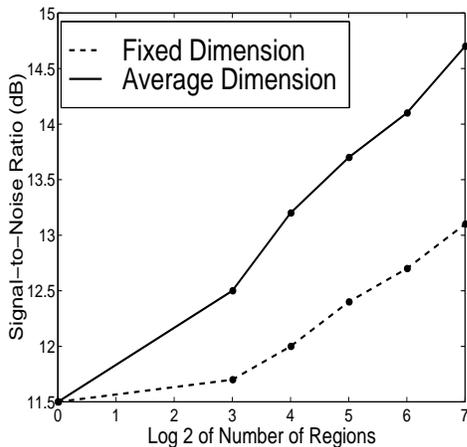
Figure 2: Dimension reduction of image blocks from 64 to 8 dimensions with fixed local dimension (dashed curve) and variable local dimension (solid curve).
