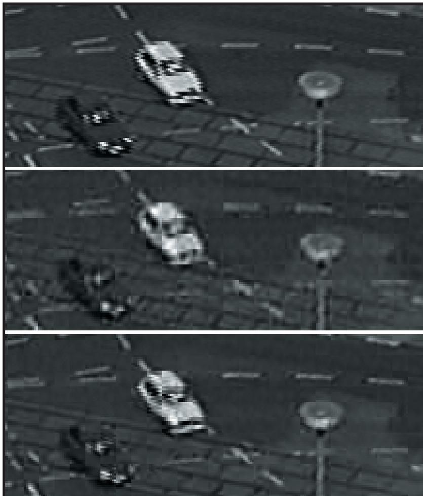
Figure 2: Sections from a test image compressed to 0.5 bpp. From top to bottom, original image, image compressed using global PCA transform coding, and CLBG transform coding with 32 regions.
