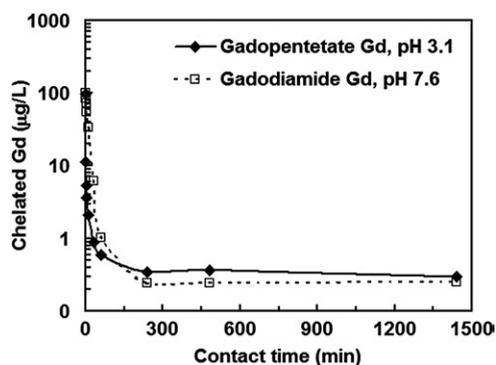
Figure 4. Adsorption kinetics of gadopentetate Gd and gadodiamide Gd measured on 1,2-HOPO-SAMMS, initial [chelated Gd] of 100  $\mu\text{g/L}$ , L/S of 5000 mL/g.
