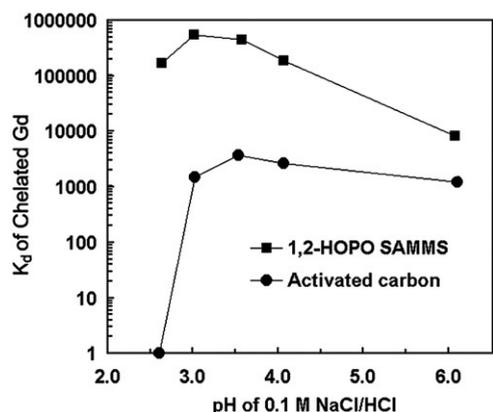
Figure 2. Distribution coefficients of gadopentetate Gd measured on 1,2-HOPO-SAMMS and Darco KB-B activated carbon in pH-adjusted 0.1 M NaCl, initial [gadopentetate Gd] of 50 ppb and L/S of 5000 mL/g.
