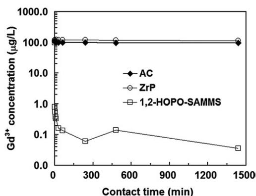
Figure 3. Adsorption kinetics of  $\text{Gd}^{3+}$  measured on 1,2-HOPO-SAMMS, activated carbon (AC), and zirconium phosphate (ZrP) in dialysate (pH 8.0), initial [ $\text{Gd}^{3+}$ ] of 100  $\mu\text{g/L}$ , L/S of 5000 mL/g.
