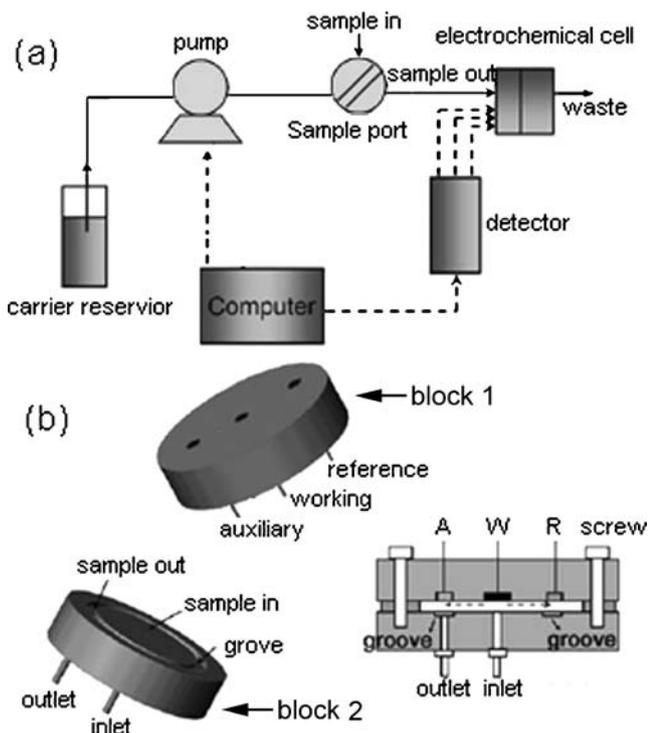
**Fig. 1a, b** Schematics of the metal analyzer (a) and the electrochemical cell (1.8 cm×2.4 cm in size ; b); solid lines represent liquid lines and dashed lines represent electronic cable lines
