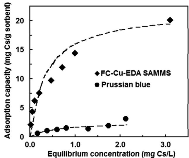
Fig. 2. Cs adsorption capacity of FC-Cu-EDA-SAMMS and Prussian blue, measured in synthetic gastric fluid (pH 1.1), L/S of 10,000 mL  $g^{-1}$ . Dashed lines represent Langmuir isotherm models.
