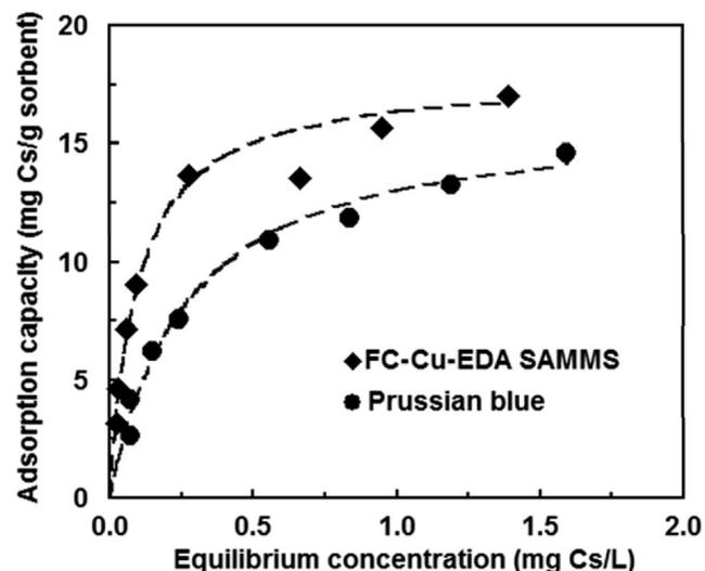
Fig. 3. Cs adsorption capacity of Cu-FC-EDA-SAMMS and Prussian blue, measured in synthetic intestinal fluid (pH 8.6), L/S of 10,000 mL g<sup>-1</sup>. Dashed lines represent Langmuir isotherm models.
