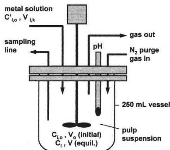
**Figure 1.** Stirred tank apparatus for fed-batch addition of Na (as NaOH or NaCl) and Ca (as CaCl<sub>2</sub>) into dilute pulp suspensions.
