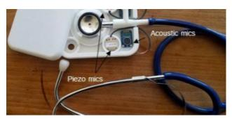
Early prototype of the "Telluscope" digital stethoscope developed by Dr. Schulman and his team.
